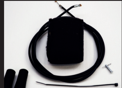
Fig 1: WISAD refurbishment consumable pack (single disconnect worth of equipment illustrated).
