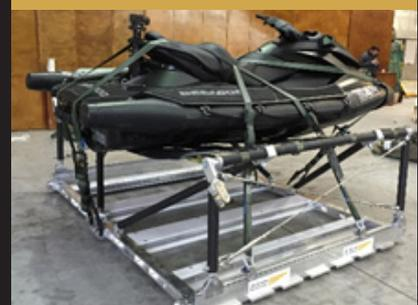
Fig 4: ATAX can be used to drop small maritime assets
