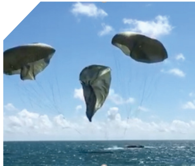
Fig 8: Parachute disconnect upon splashdown
