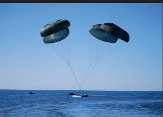
Designed for use in Special Operations and SAR missions, MCADS enable Rigid Inflatable Boats to be parachute dropped into the water, ready for immediate use.
